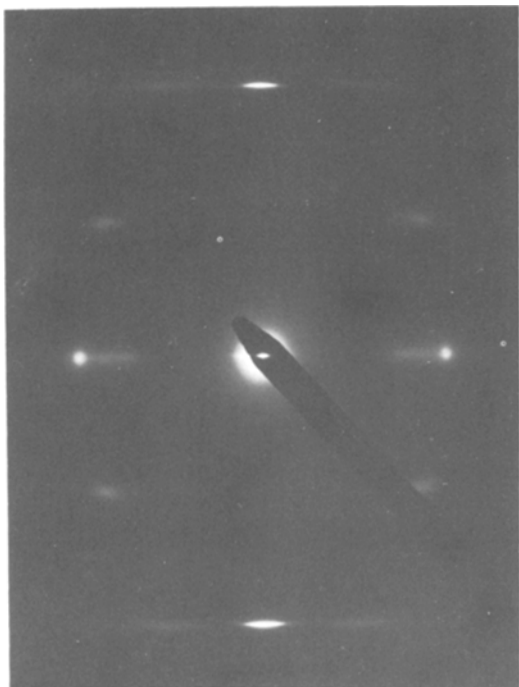
Figure 7 Electron diffraction pattern of a fibril branched from a whisker grown in the presence of camphene.
